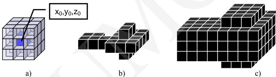
Fig. 1. Neighborhood shape used in the 3D multi-class region growing (a), example 3D region (b), example 3D region after dilation (c)
