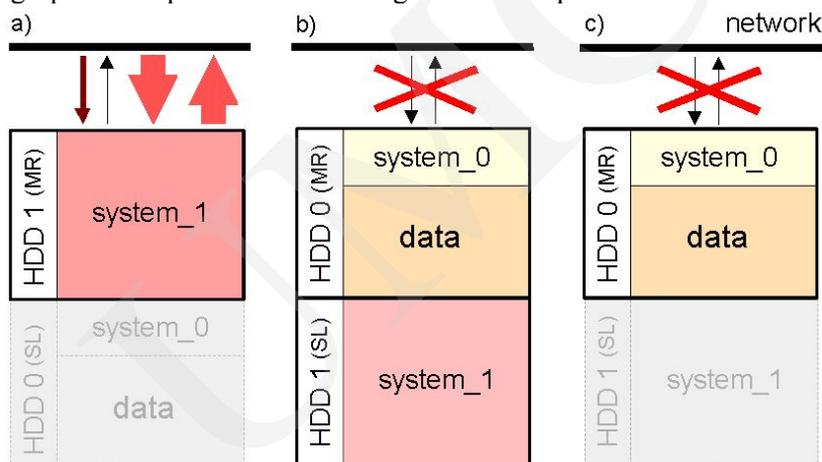
Fig. 1. Scheme of configuration of HDD disks in computer for different modes of operation: with network (a) and without network (b, c)
