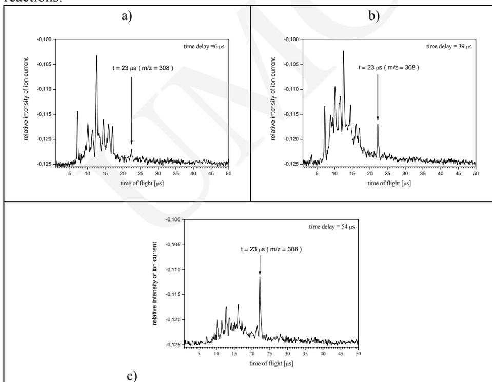
Fig. 4. Relative intensity of the ion current of 2,5-dihydroxybenzoic acid. The time delay between the laser shot and turning on the accelerating voltage: a) 6  $\mu\text{s}$ , b) 39  $\mu\text{s}$ , c) 54  $\mu\text{s}$
