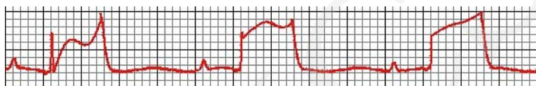
Fig. 6. An example with the ST segment modification. For the comparison the base signal is presented in Fig. 4.
