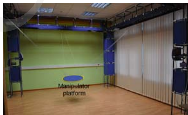
Fig. 5. The photo of described cable-driven manipulator.
